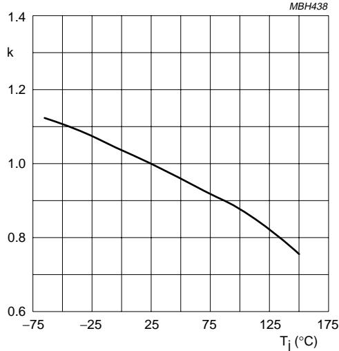
$$k = \frac{V_{GS\text{th}} \text{ at } T_j}{V_{GS\text{th}} \text{ at } 25^\circ\text{C}}$$
