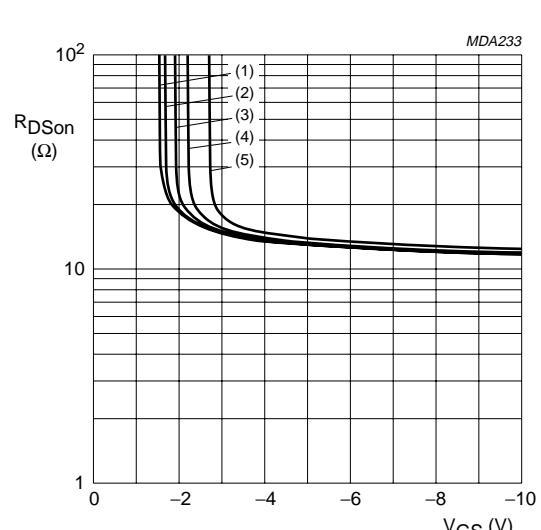
$V_{DS} \geq I_D \times R_{DSon}; T_{amb} = 25$  °C;  $t_p = 300$  μs;  $\delta = 0$ .
