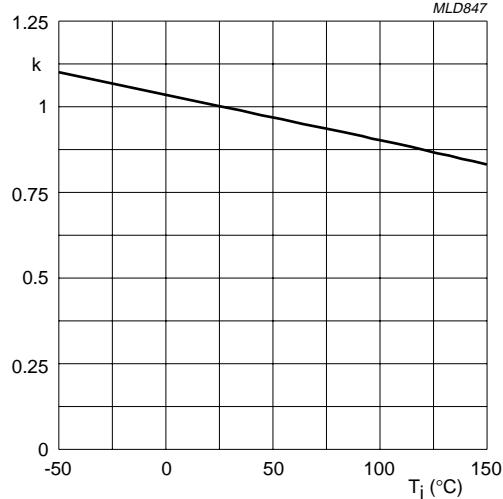
$$k = \frac{V_{GS\text{th}} \text{ at } T_j}{V_{GS\text{th}} \text{ at } 25^\circ\text{C}}$$
