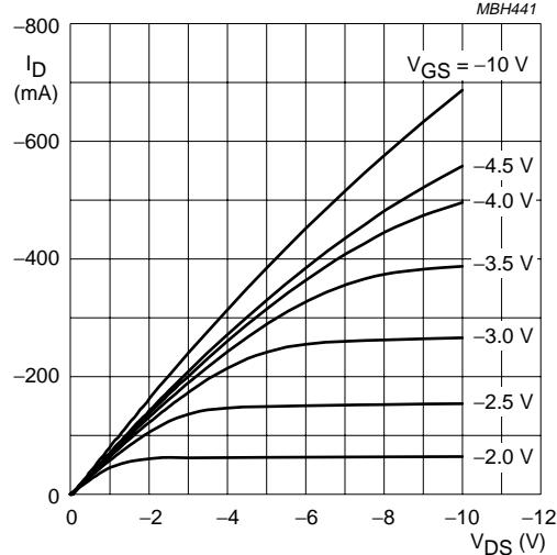
$T_{amb} = 25 \text{ }^{\circ}\text{C}; t_p = 80 \mu\text{s}; \delta = 0.$
