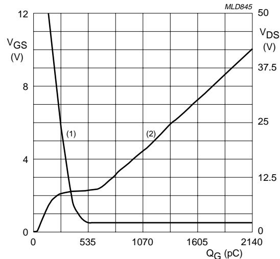
$V_{\text{DD}} = -50 \text{ V}; I_{\text{D}} = -115 \text{ mA}; T_{\text{amb}} = 25^\circ\text{C}.$ (1) V<sub>DS</sub>. (2) V<sub>GS</sub>.
