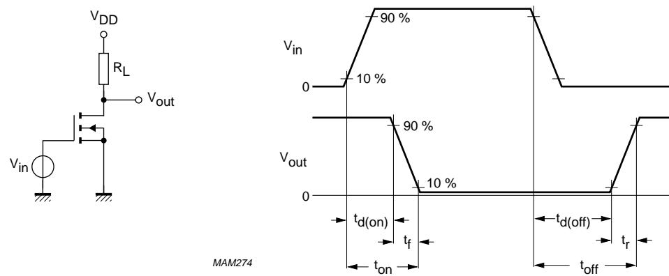
Fig.6 Switching times test circuit with input and output waveforms; N-channel.
