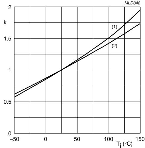
$$k = \frac{R_{DSon} \text{ at } T_j}{R_{DSon} \text{ at } 25^\circ\text{C}}$$
