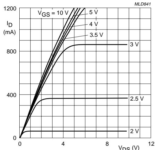
$T_{amb} = 25 \text{ }^{\circ}\text{C}; t_p = 80 \mu\text{s}; \delta = 0.$
