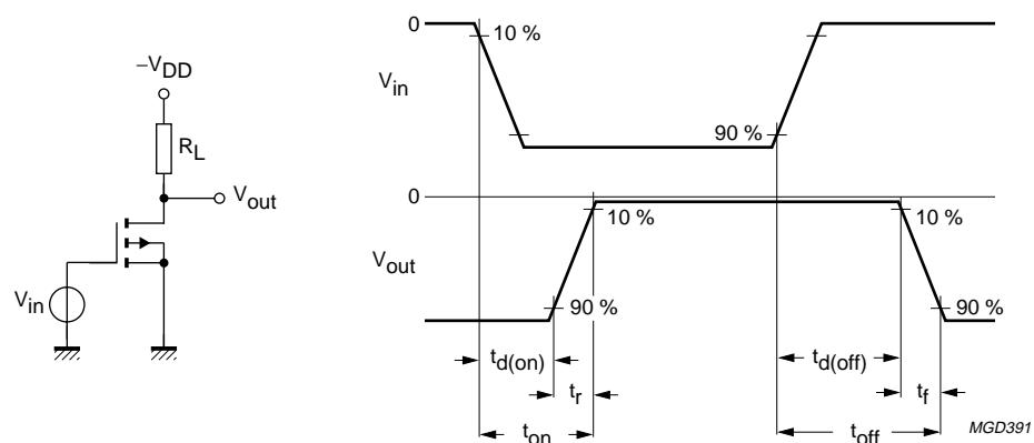
Fig.7 Switching times test circuit with input and output waveforms; P-channel.
